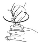
**18** Push down "T" plunger and move plunger in a circular motion to further puncture the foil seal so fluid can be poured out.
