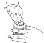
**19** Remove flexible cap and drainage line from bottle.
